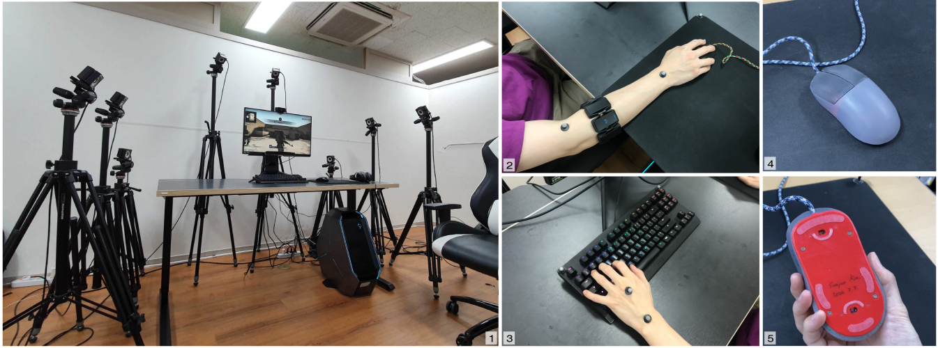
Figure 2: Experimental setup of the gameplay logging system: Box 1 shows the desktop setup of eight motion-capture cameras. Boxes 2 and 3 are the positions of the reflective markers and MYO armband. Boxes 4 and 5 are the dual-sensor mouse and two sensor positions. The ear-clip type pulse sensor was attached to the player’s right earlobe (not pictured).
